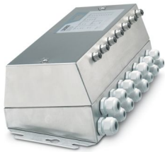
Electronic motor starter, 3.0 kW, single-channel, IP67 degree of protection
