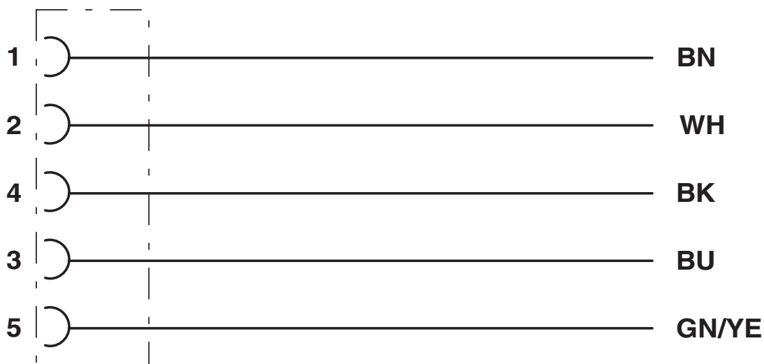
Contact assignment of the M12 sockets
