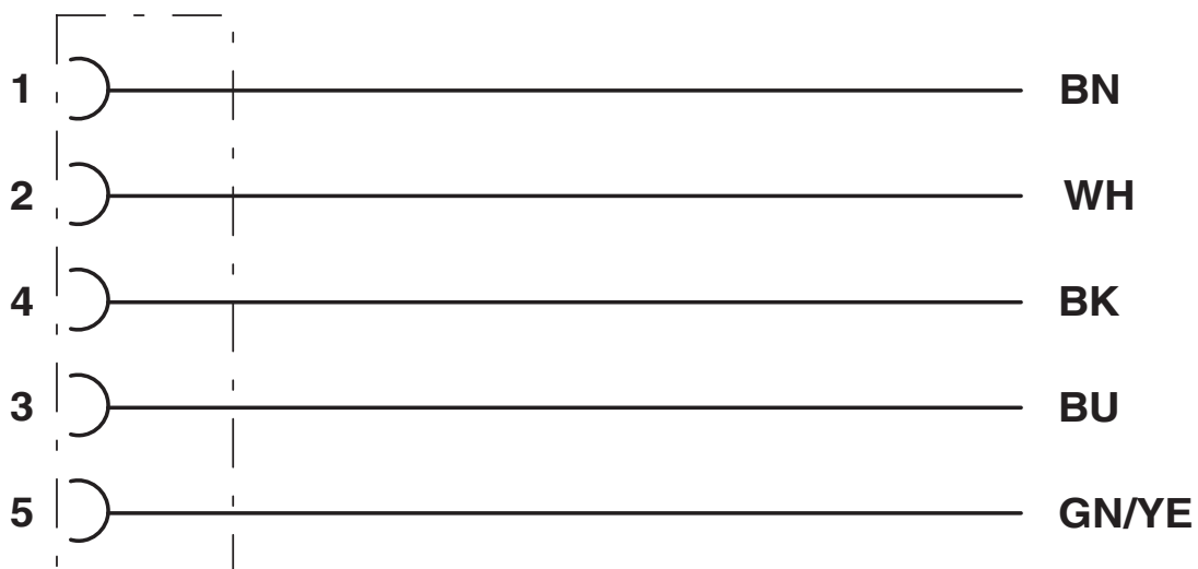
Contact assignment of the M12 sockets
