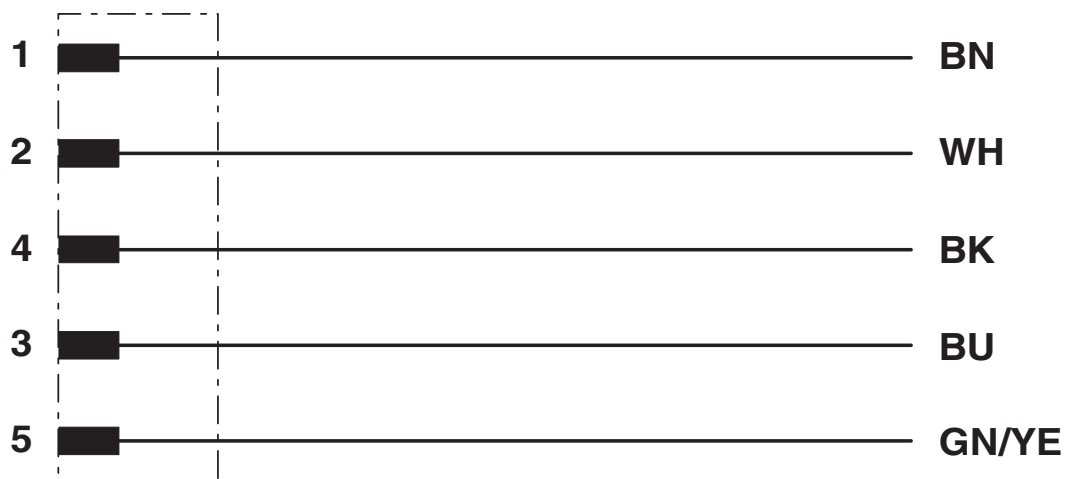
Contact assignment of the M12 plug
