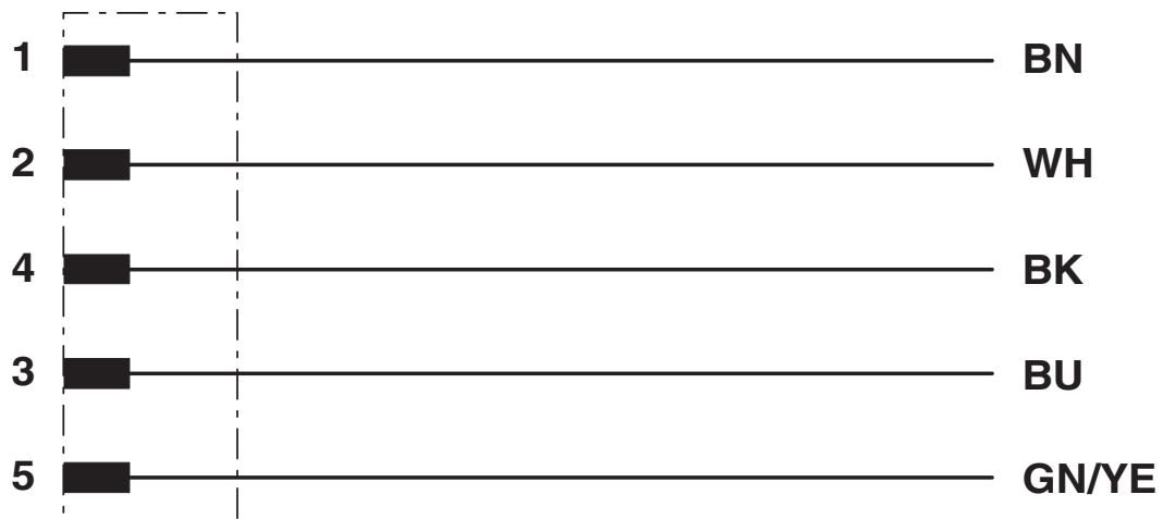
Contact assignment of the M12 plug
