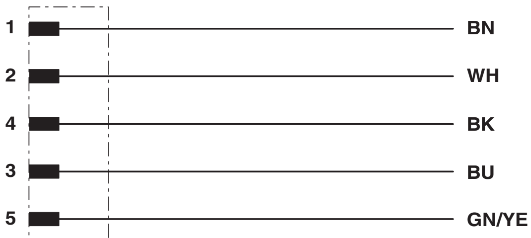
Contact assignment of the M12 plug
