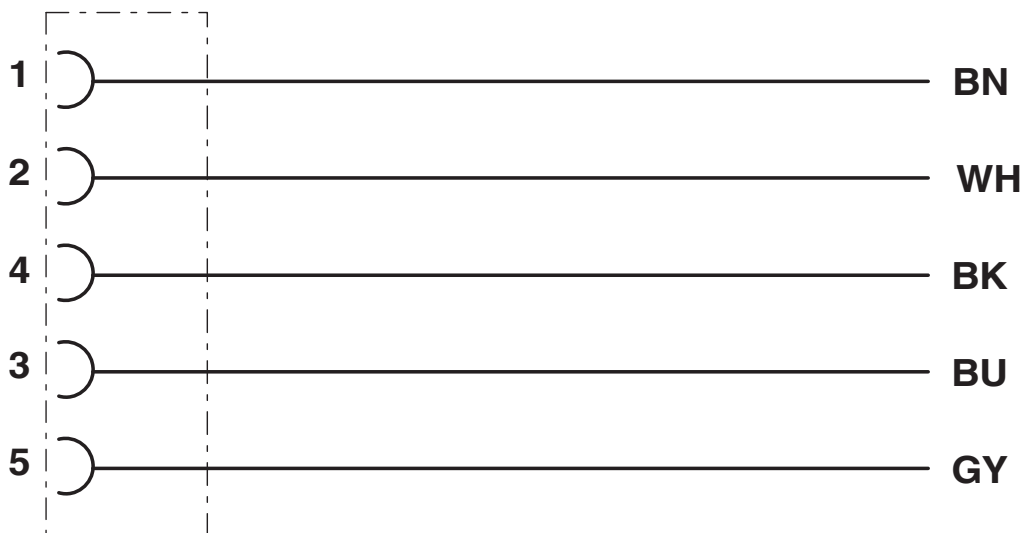
Contact assignment of the M12 socket
