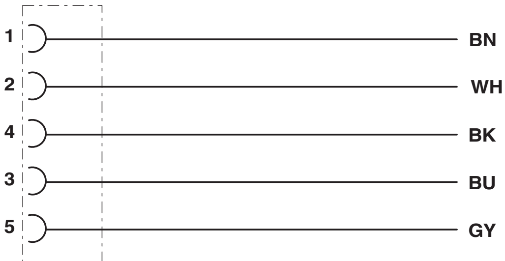
Contact assignment of the M12 socket
