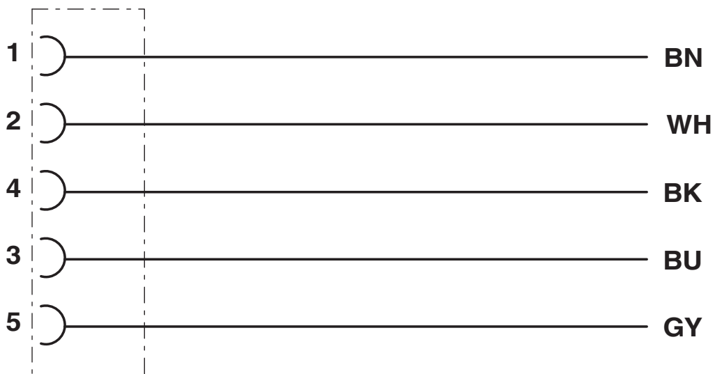
Contact assignment of the M12 socket
