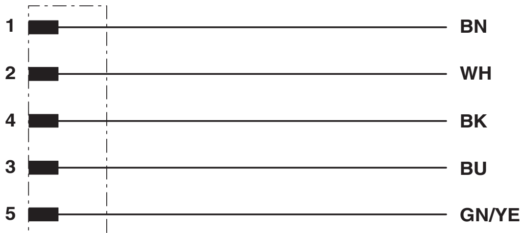
Contact assignment of the M12 plug
