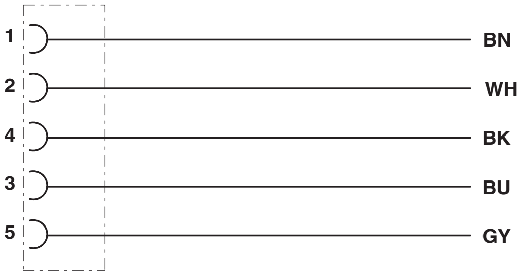
Contact assignment of the M12 socket
