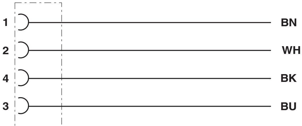
Contact assignment of the M12 socket
