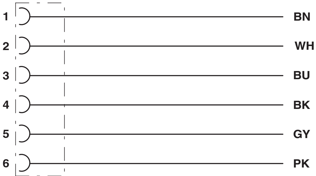
Contact assignment of M8 socket
