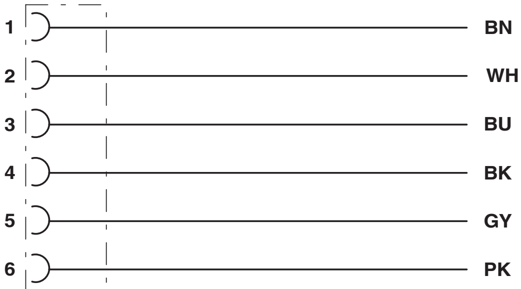
Contact assignment of M8 socket
