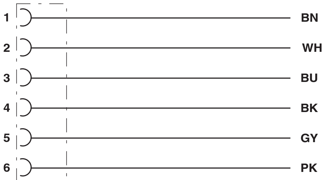
Contact assignment of M8 socket
