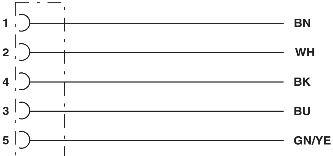
Contact assignment of the M12 socket
