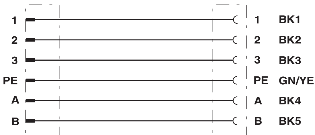
Contact assignment of the S15 plug and the S15 socket
