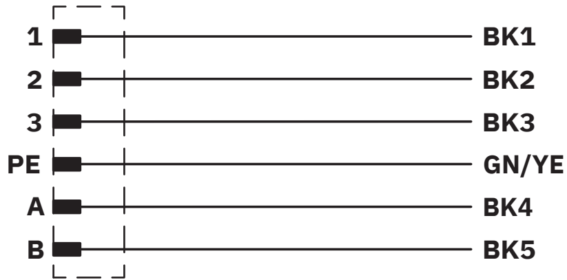
Contact assignment of the M15 connector
