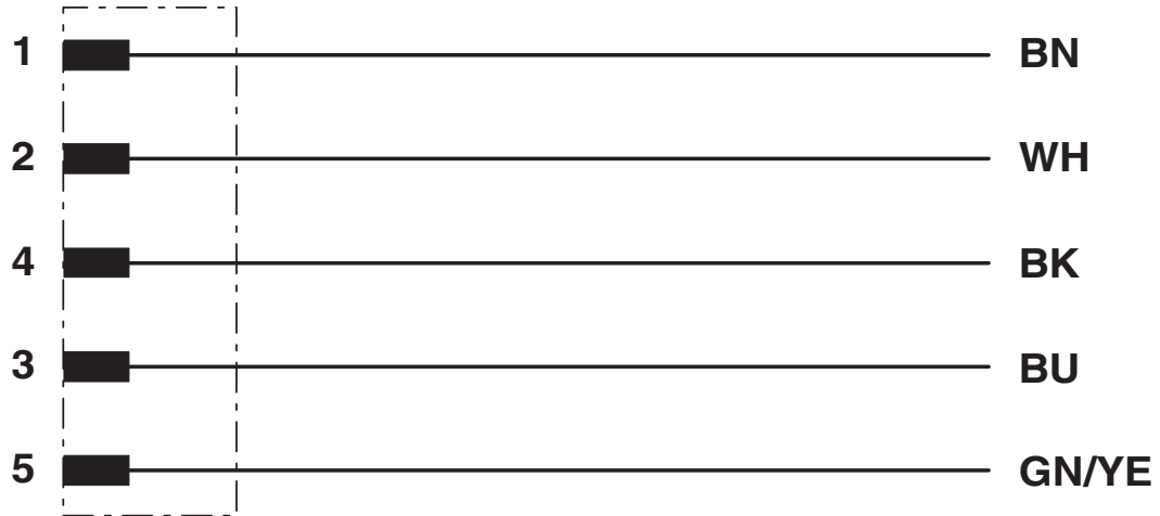
Contact assignment of the M12 plug
