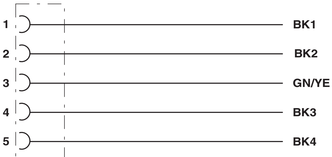
Contact assignment of 7/8" socket
