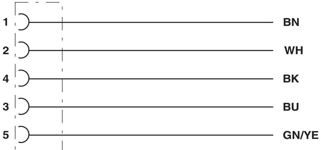
Contact assignment of the M12 sockets
