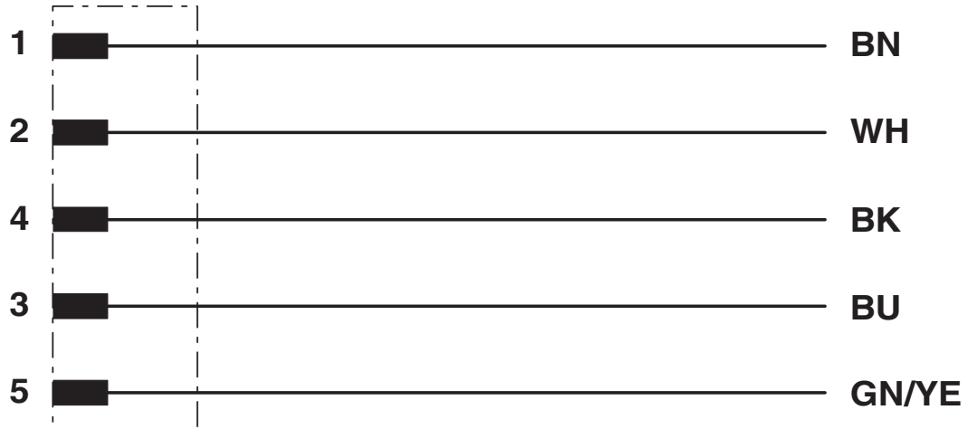
Contact assignment of the M12 plug
