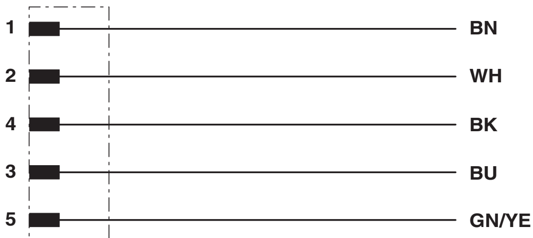
Contact assignment of the M12 plug
