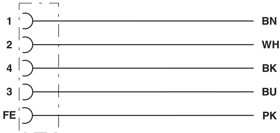
Contact assignment of the M12 socket
