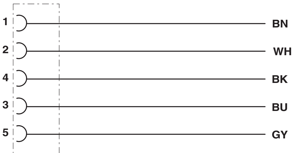
Contact assignment of the M12 socket
