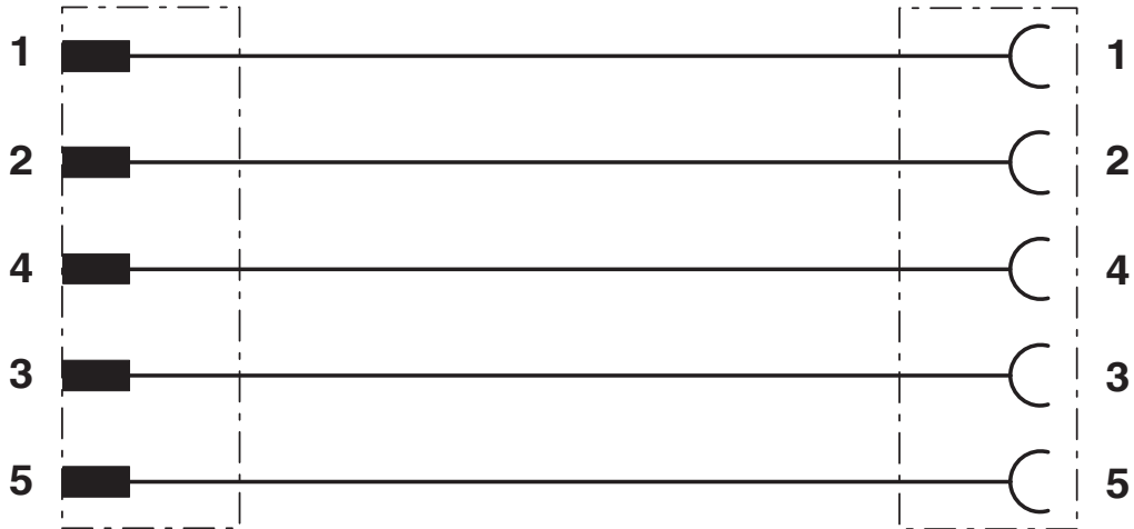
Contact assignment of M8 plugs/sockets
