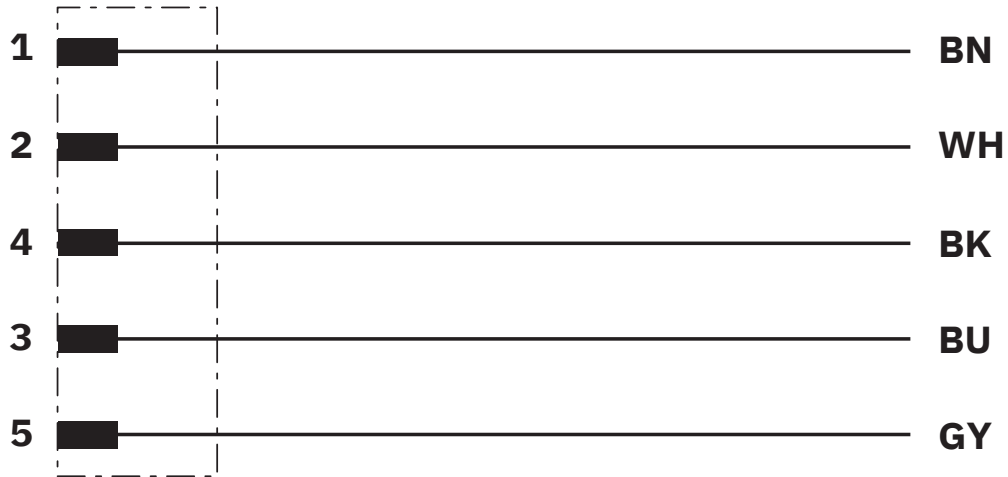
Contact assignment of the M12 plug
