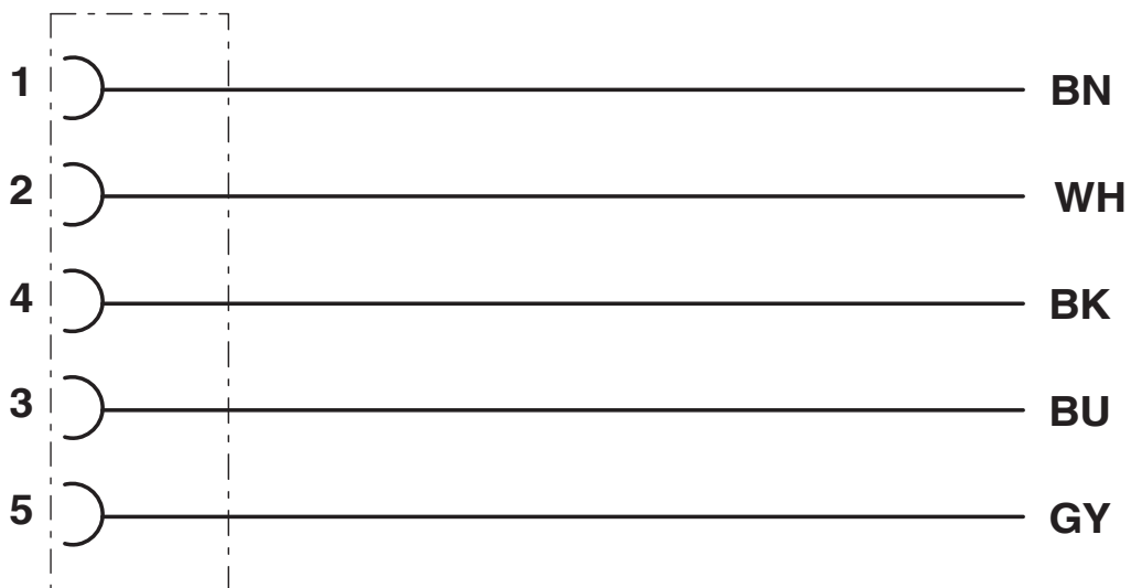
Contact assignment of the M12 socket
