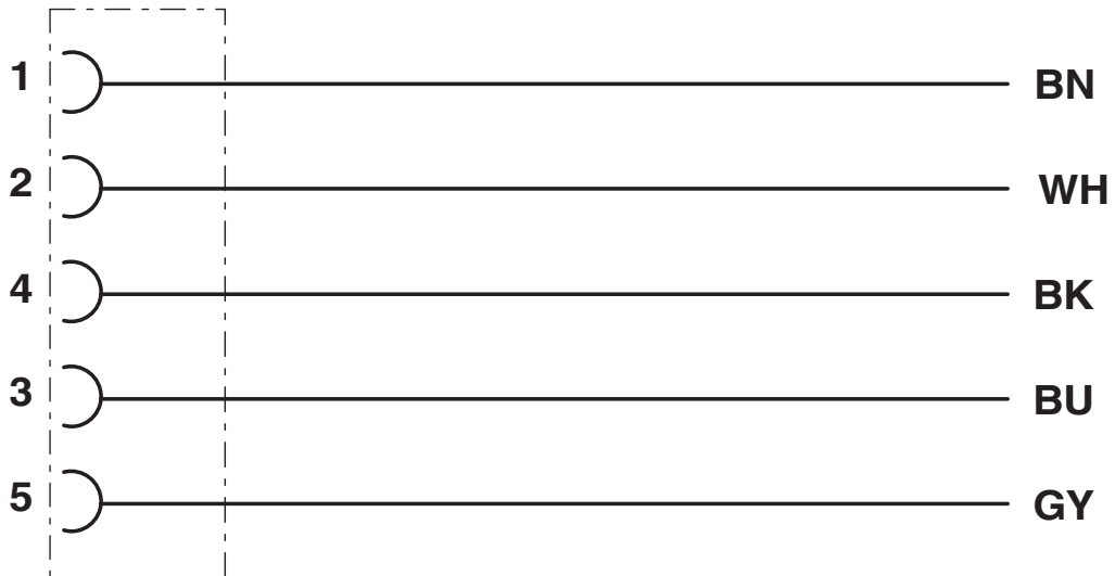
Contact assignment of the M12 socket
