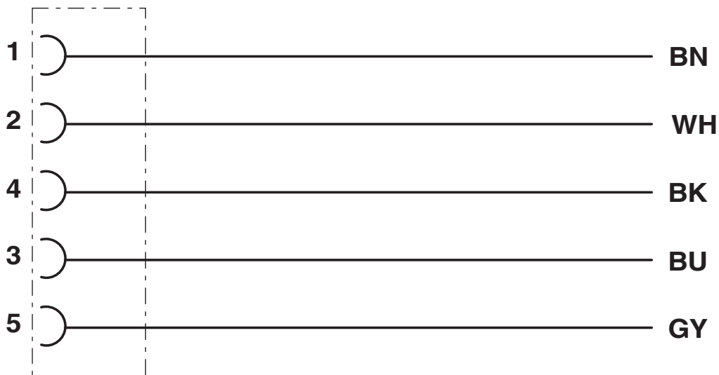
Contact assignment of the M12 socket
