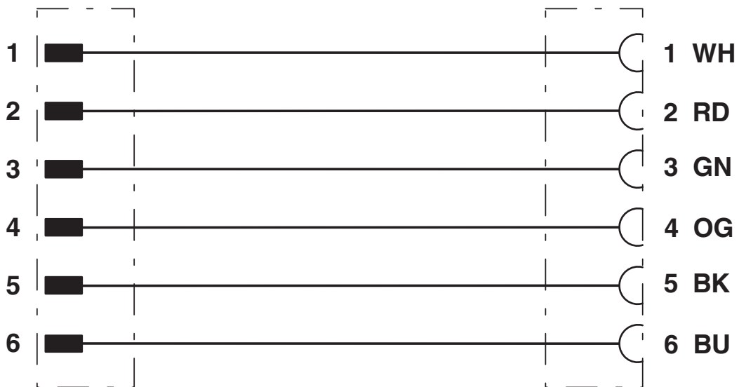
Contact assignment of 7/8" plugs/sockets
