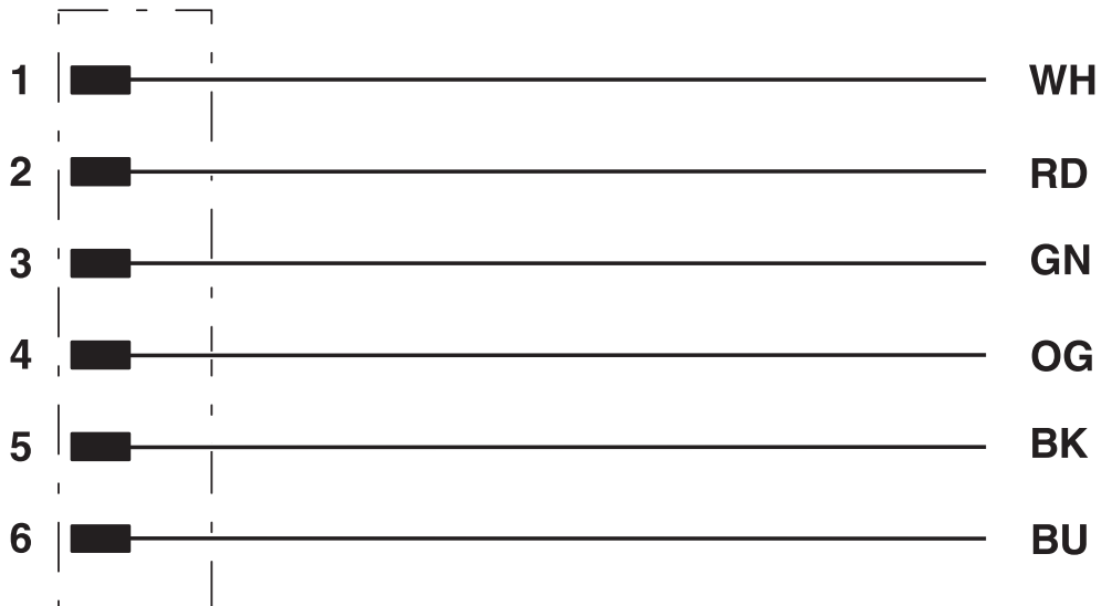
Contact assignment of 7/8" plug
