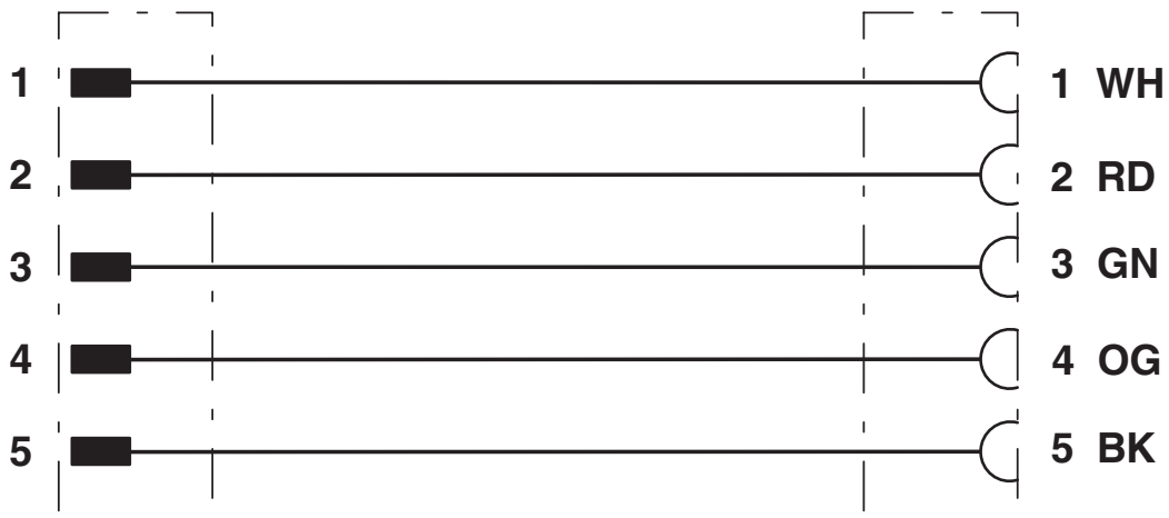
Contact assignment of 7/8" plugs/sockets
