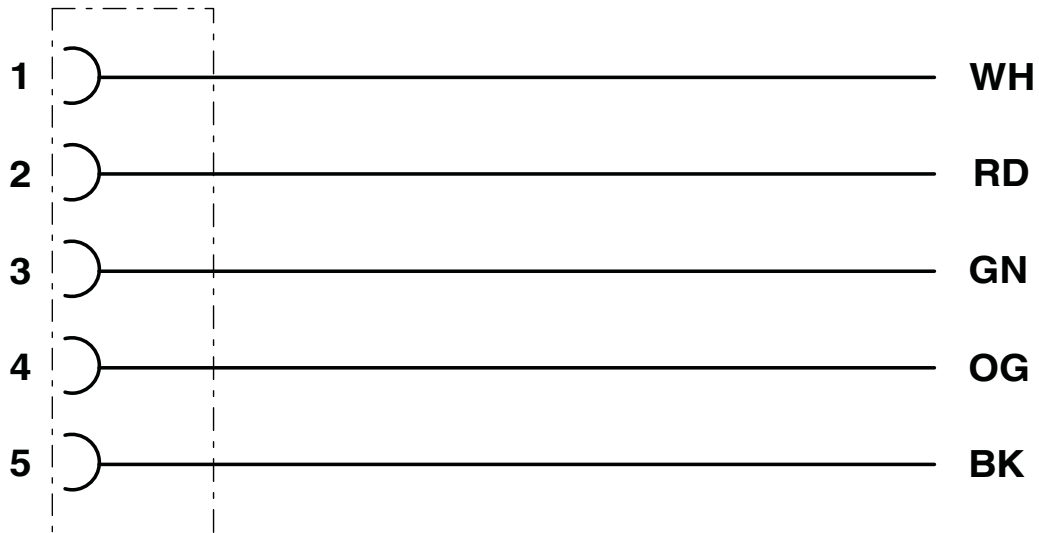
Contact assignment of 7/8" socket
