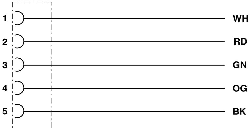
Contact assignment of 7/8" socket
