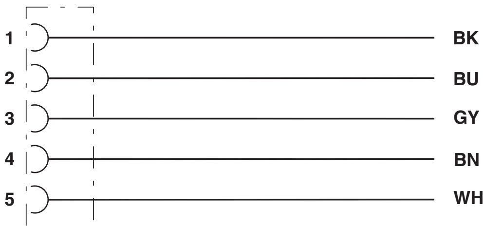
Contact assignment of 7/8" socket
