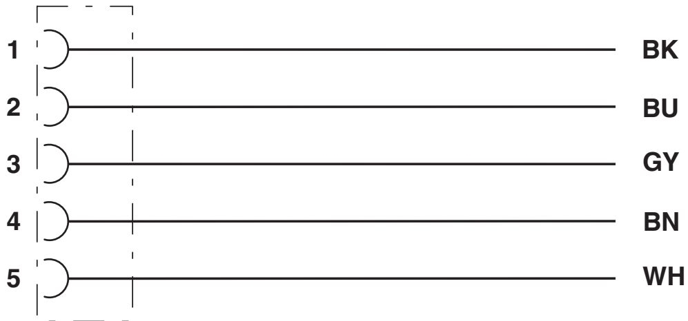
Contact assignment of 7/8" socket
