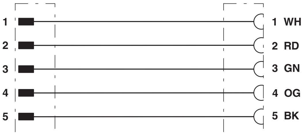
Contact assignment of 7/8" plugs/sockets
