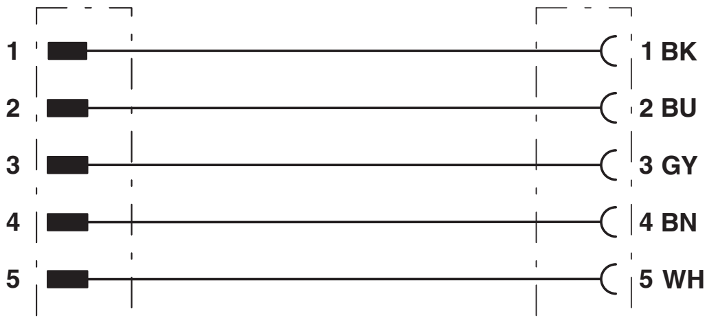
Contact assignment of 7/8" plugs/sockets
