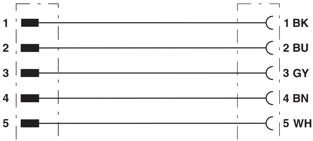
Contact assignment of 7/8" plugs/sockets
