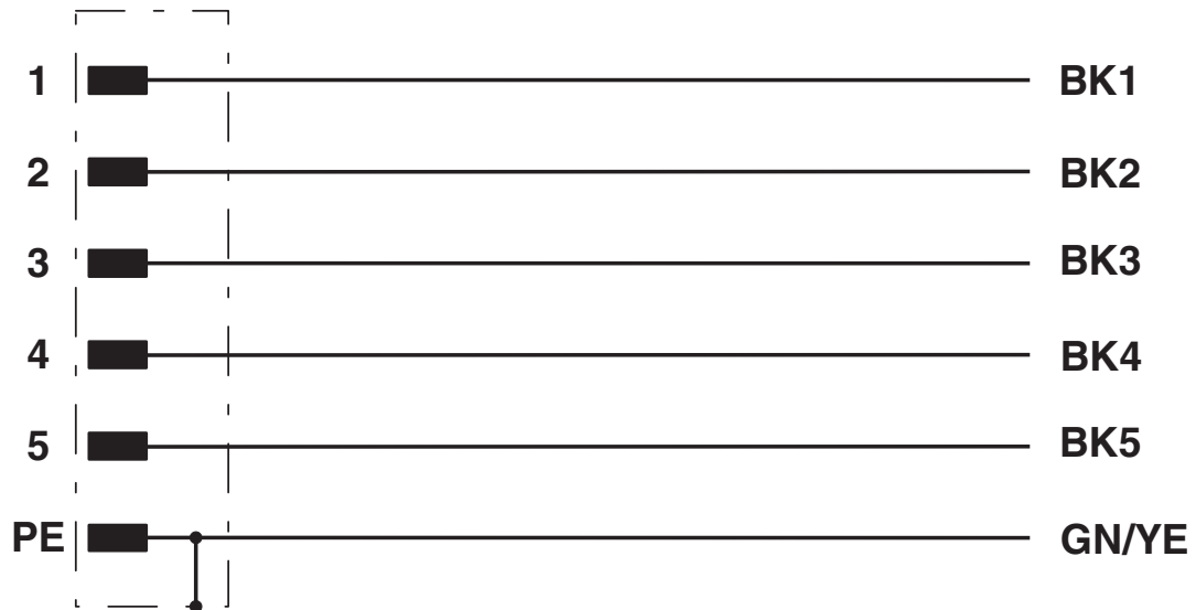
Contact assignment of the M12 plug
