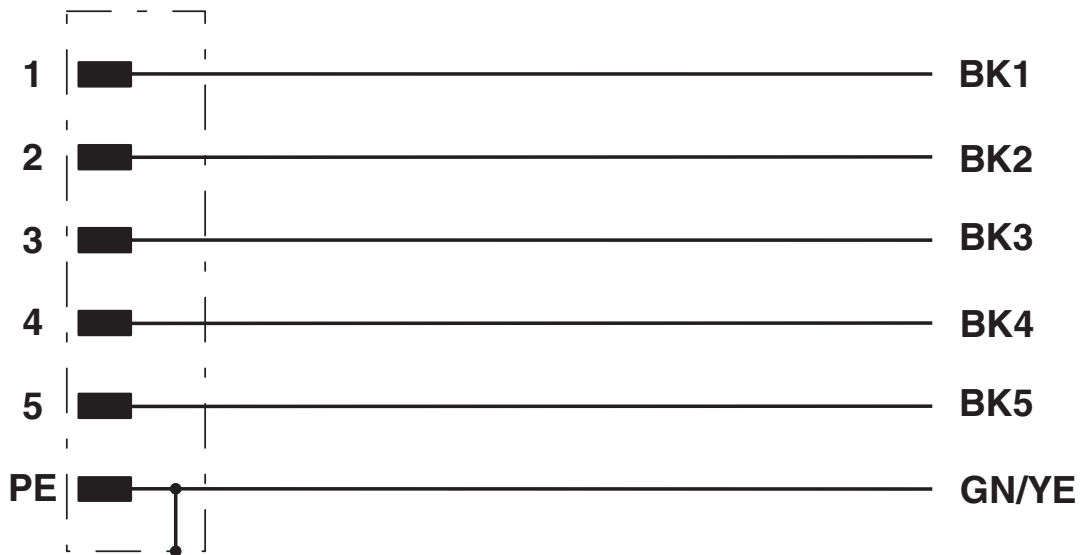
Contact assignment of the M12 plug
