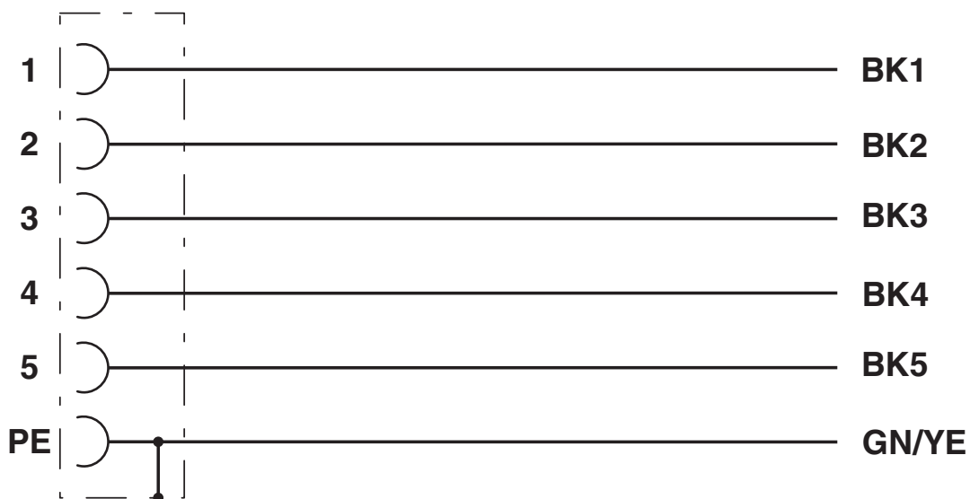
Contact assignment of the M12 socket
