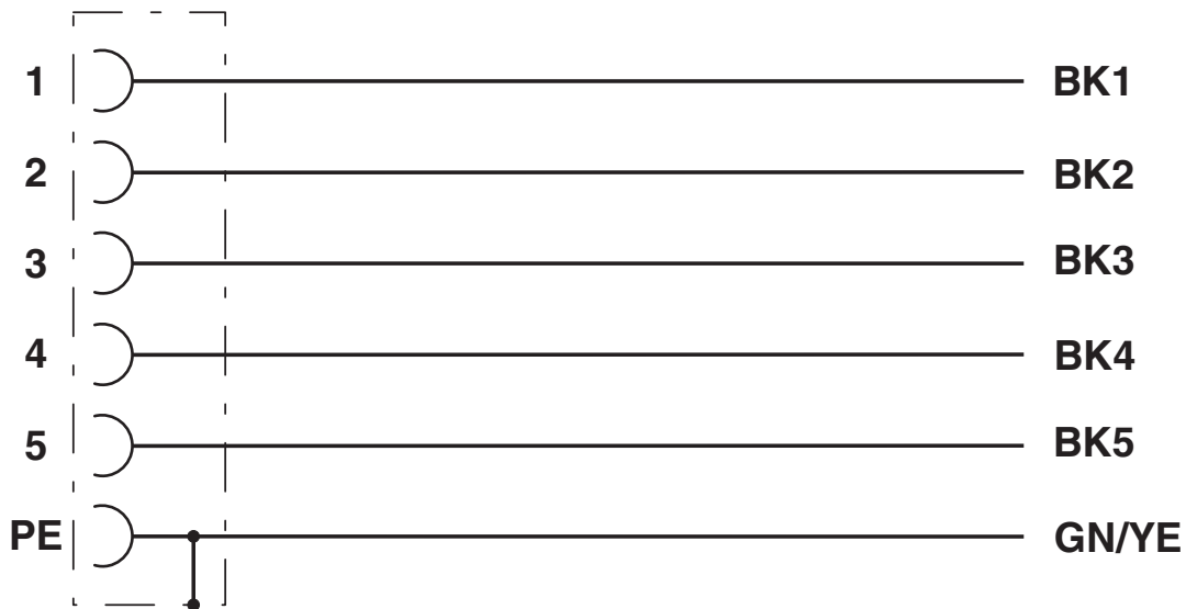
Contact assignment of the M12 socket
