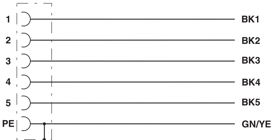
Contact assignment of the M12 socket
