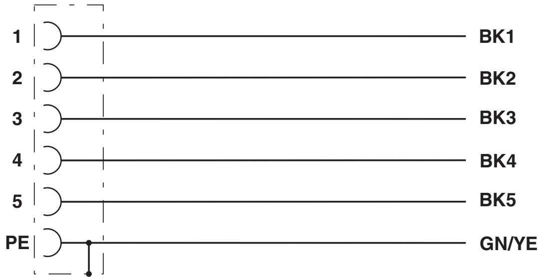
Contact assignment of the M12 socket
