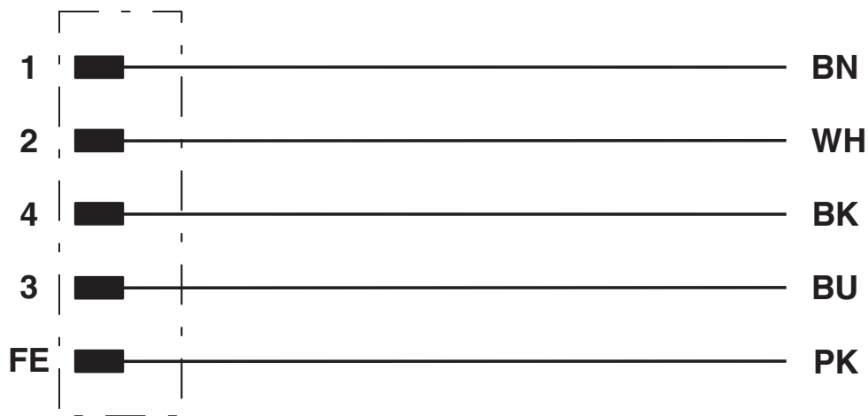
Contact assignment of the M12 plug
