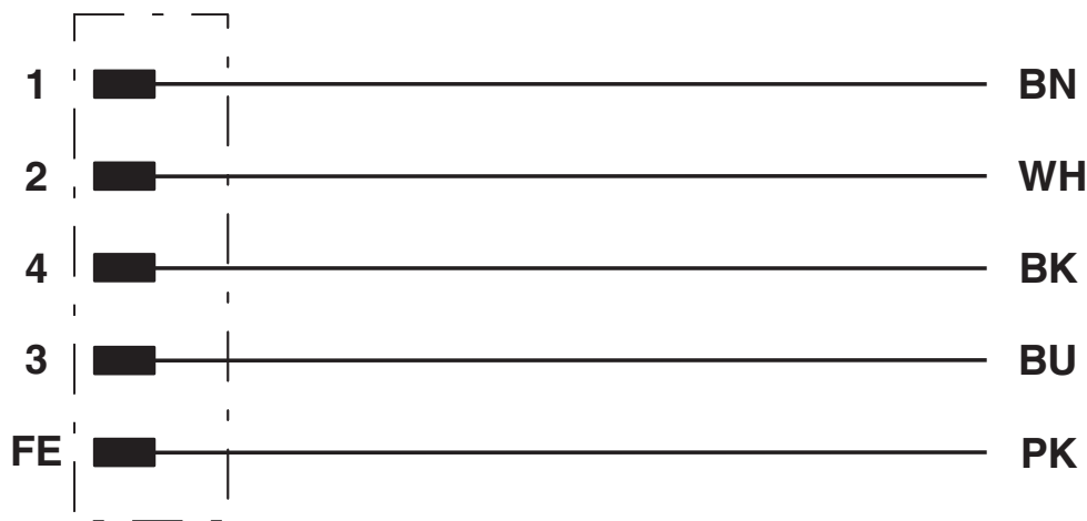
Contact assignment of the M12 plug
