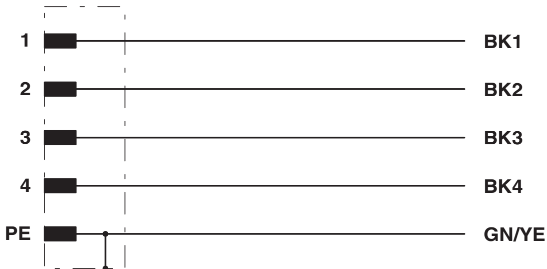
Contact assignment of the M12 plug
