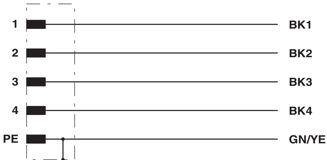
Contact assignment of the M12 plug
